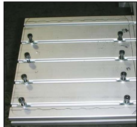
**NOTE 1:** The screws are different lengths; the eight screws toward the front of the machine are longer than the eight screws toward the rear. (PICTURE 9)
